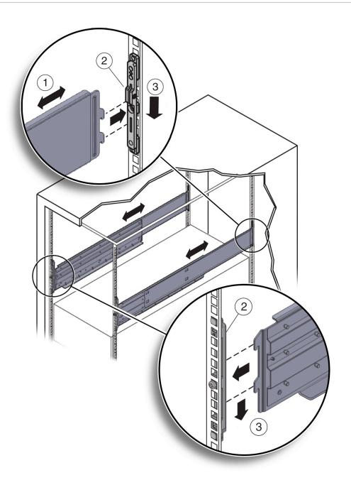
8. Thread the four M4 x 10 flathead locking screws into the four adapter brackets [1]).
