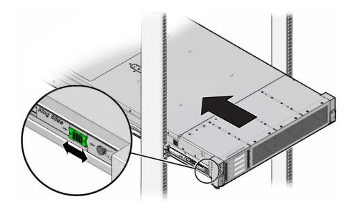
c. Continue pushing the server into the rack until the slide-rail locks (on the front of the server) engage the slide-rail assemblies.
