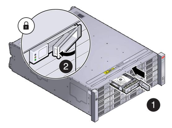
Once installed, the system should automatically detect and use the replacement drive. Ensure that the green OK indicator for the replacement drive lights to show that the drive is ready.
