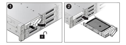
4. Align the replacement drive with the drive slot.
