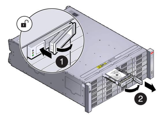
**3.** Install the replacement drive by opening the drive lever on the replacement drive. Slide the new drive into the drive slot [1] until it engages with the backplane connector and then close the lever to fully seat the drive and lock it into place [2] as shown in the following figure.
