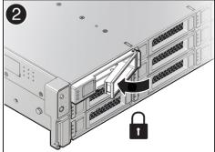
6. Power on and remount the replacement drive. Type the following command from the host:
