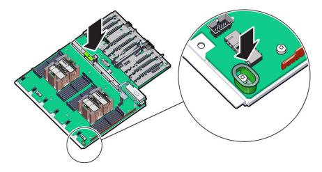
**b.** Carefully slide the motherboard forward, and while holding the motherboard mid-wall handle and small plastic motherboard handle, lift it out of the chassis.
