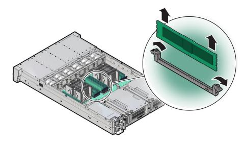
Replace each failed DIMM with either another DIMM of the same rank size (quad-rank or dual-rank) or leave the slot empty.
