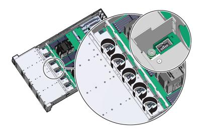
4. Install the fan modules into the fan tray.
