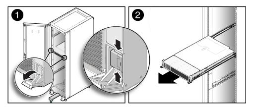
4. While the release latch covers are in the open position, slowly pull the server forward until the slide-rails latch into a locked position [2].
