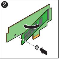
b. With the M.2 flash SSD at an approximate 45 degree angle to the riser board, insert the plastic retainer clip into the notched end of the M.2 flash SSD and then push down on the end of the M.2 flash SSD until the retainer clip snaps into place in the hole on the riser board [2].
