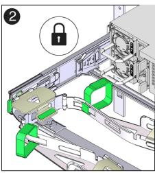
**8.** Gently tug on the four CMA connection points to ensure that the CMA connectors are fully seated before you allow the CMA to hang by its own weight.
