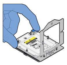
Lift the processor rail frame by holding its lift tabs and rotating the rail frame to its near vertical position.
