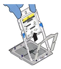
Retain the external cap. Do not attempt to reinstall it. The cap will need to be placed on the processor socket of the old motherboard. This will prevent damage during shipping back to the Service Center for motherboard failure analysis.
