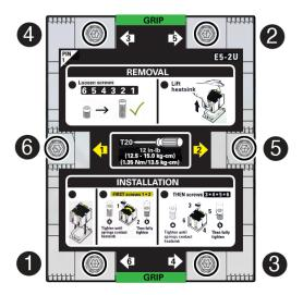
4. Lift the heatsink from the socket.
