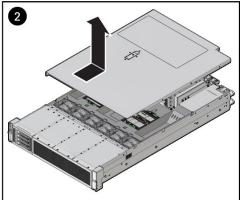
4. Lift up and remove the top cover [2].
