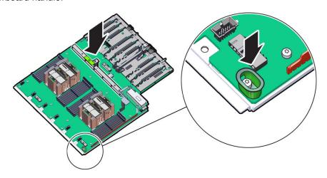
**b.** Carefully slide the motherboard forward, and while holding the motherboard mid-wall handle and small plastic motherboard handle, lift it out of the chassis.
