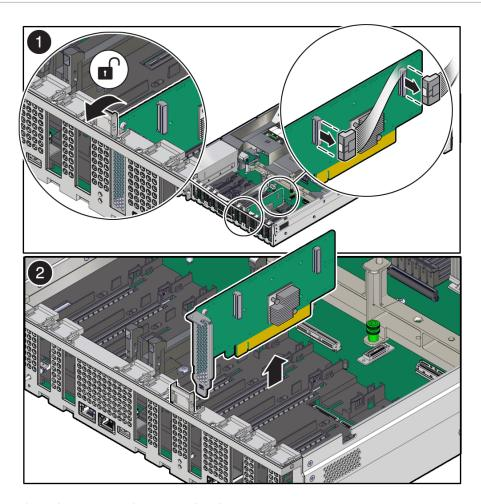
6. Place the PCIe card on an antistatic mat.
