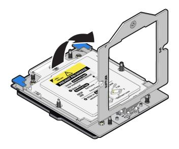
c. On the socket, open the Rail Frame.
