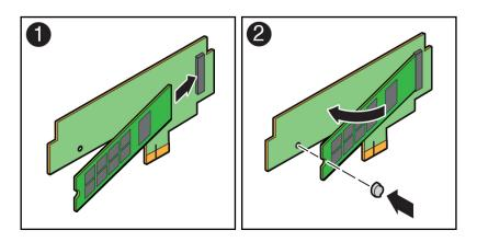
b. With the M.2 flash SSD at an approximate 45 degree angle to the riser board, insert the plastic retainer clip into the notched end of the M.2 flash SSD and then push down on the end of the M.2 flash SSD until the retainer clip snaps into place in the hole on the riser board [2].
