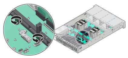
**10.** Remove the motherboard from the server with reusable components that populate the motherboard in place.
