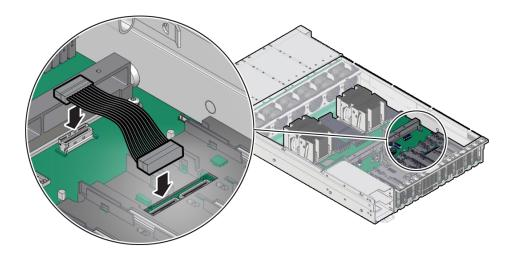
Plug each end of the cable into its connector until you hear an audible click.
