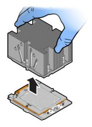
5. Place the heatsink, facing up, on a work surface.
