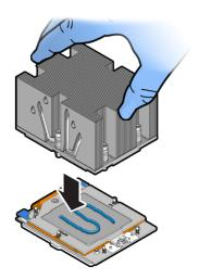
9. Using torque driver set to 12 in-lb (13.5 kg-cm) to 13.02 in-lb (15.0 kg-cm) force with a Torx T20 bit, tighten the heatsink module to the socket as shown in the following illustration. Note that screws 1 and 2 are slightly longer than screws 3, 4, 5, and 6.
