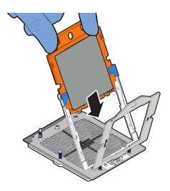
Ensure that the two insertion tabs at the bottom of the processor carrier are inserted into the tab slots in the Rail Frame.
