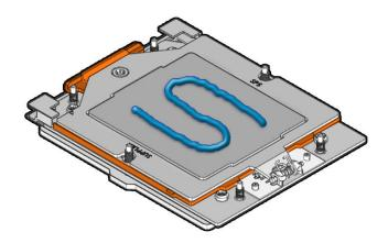
8. Carefully lower the heatsink on to the six socket heatsink attachment studs.
