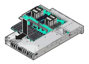
3. Using a Torx T25 screwdriver, tighten the two captive screws to secure the motherboard mid-wall to the chassis.
