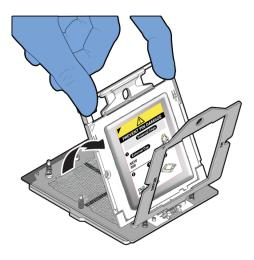
**d.** Holding the socket cover external cap by its handle, slide the External Cap up and out of the Rail Frame.
