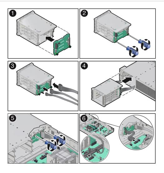
b. Reconnect the disk backplane cables to the disk backplane [3].
