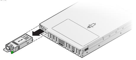
7. Pull the power supply out of the chassis.
