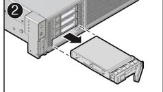
4. Align the replacement drive with the drive slot.
