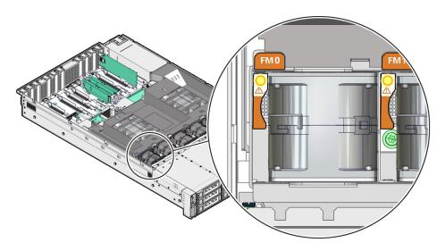
4. Using your forefinger and thumb, lift the fan module straight up and out of the chassis and set it aside on an antistatic mat.
