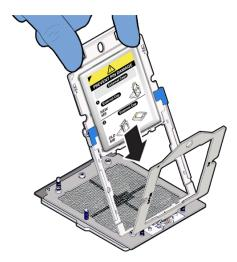
Ensure that the two insertion tabs at the bottom of the External Cap are inserted into the slots in the rail frame.
