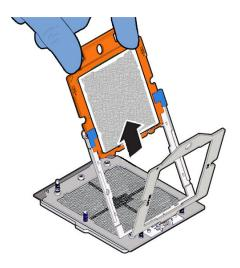
**12.** Place the carrier frame package in an appropriate tray.
