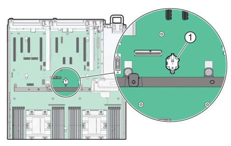
3. Remove the battery from the battery connector.
