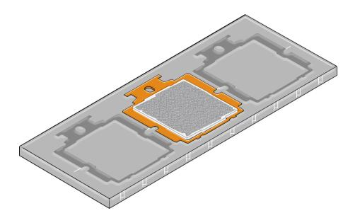
13. Wipe the Force Frame (retention frame) with a dry wipe followed by a wipe with a small amount of isopropyl alcohol.
