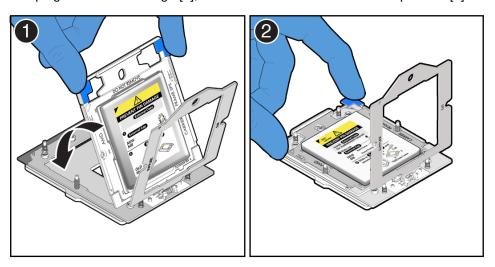
c. Rotate the force frame to its closed position on the socket stiffener frame.
