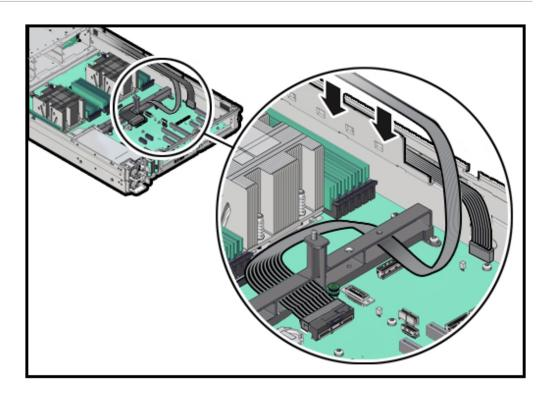
3. Reconnect the "Y" end of the Retimer cable to the Retimer card in PCIe slot 6.
