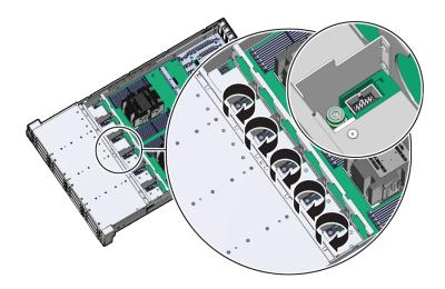
4. Install the fan modules into the fan tray.
