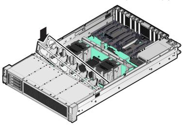
3. Using a Torx T25 screwdriver, tighten the five spring-mounted screws that secure the fan tray to the server chassis.
