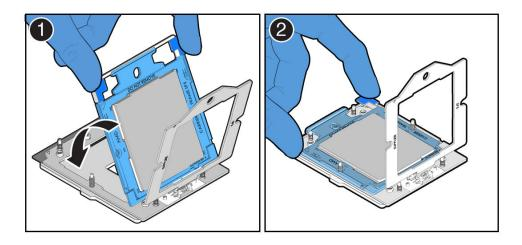
5. Rotate the Force Frame down to its closed position on the socket stiffener frame.
