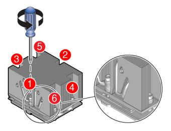
Loosen in reverse order 6-1, then go back and disengage completely.
