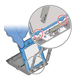
4. Grasping the Rail Frame edge [1], rotate the Rail Frame down to the closed position [2].
