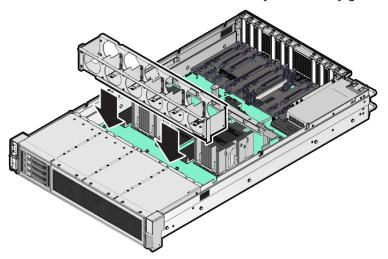
2. When installing the fan tray, the fan tray should first be slightly tilted to the left to compress the cables, before the operation.
