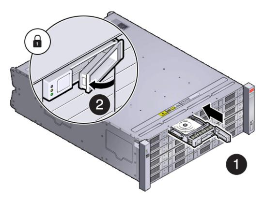
4. Once installed, the system should automatically detect and use the replacement drive. Ensure that the green OK indicator for the replacement drive lights to show that the drive is ready.
