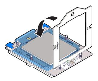
6. Using a torque driver set to 12 in-lb (inch-pound) or 1.35 Nm/13.5 kg-cm force with a Torx T20 bit, fully tighten the captive screw that secures the Force Frame to the socket stiffener frame.
