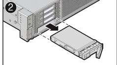
4. Align the replacement drive with the drive slot.
