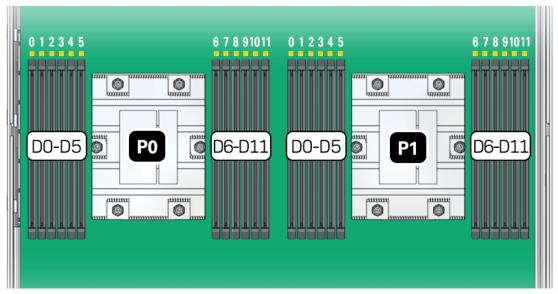
Each processor, P0 and P1, has twelve DIMM slots (D0-D11), six on each processor side. Each DIMM slot supports a single memory channel, for total of twelve DDR5 memory channels per processor (0-11).
