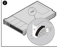
2. Latch the top cover closed by pushing down on the button until it is flush with the cover and you hear an audible click [2].
