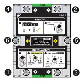
4. Lift the heatsink from the socket.
