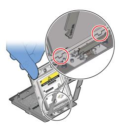
b. Grasping the rail frame edge [1], rotate the rail frame to the closed position [2].
