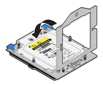
d. Using a torque driver set to 12 in-lb (inch-pound) (1.35 Nm/13.5 kg-cm) with a Torx T20 bit, fully tighten the captive screw that secures the force frame to the socket stiffener frame.
