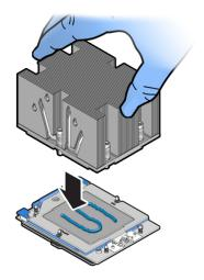
9. Using torque driver set to 12 in-lb (13.5 kg-cm) to 13.02 in-lb (15.0 kg-cm) force with a Torx T20 bit, tighten the heatsink module to the socket as shown in the following illustration. Note that screws 1 and 2 are slightly longer than screws 3, 4, 5, and 6.
