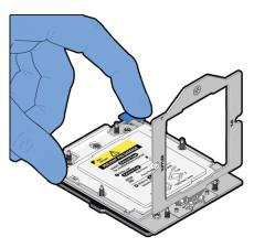
Lift the processor rail frame by holding its lift tabs and rotating the rail frame to its near vertical position.
