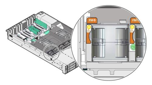
4. Using your forefinger and thumb, lift the fan module straight up and out of the chassis and set it aside on an antistatic mat.
