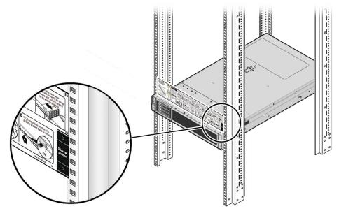
4. Mark the mounting holes for the back slide-rails.
