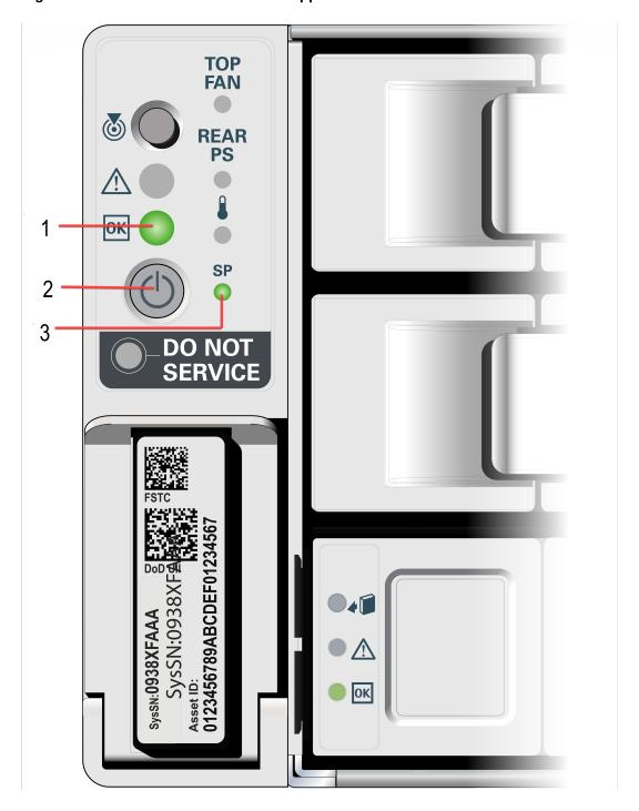
Figure 3-1 Front of Oracle Database Appliance Power Panel
