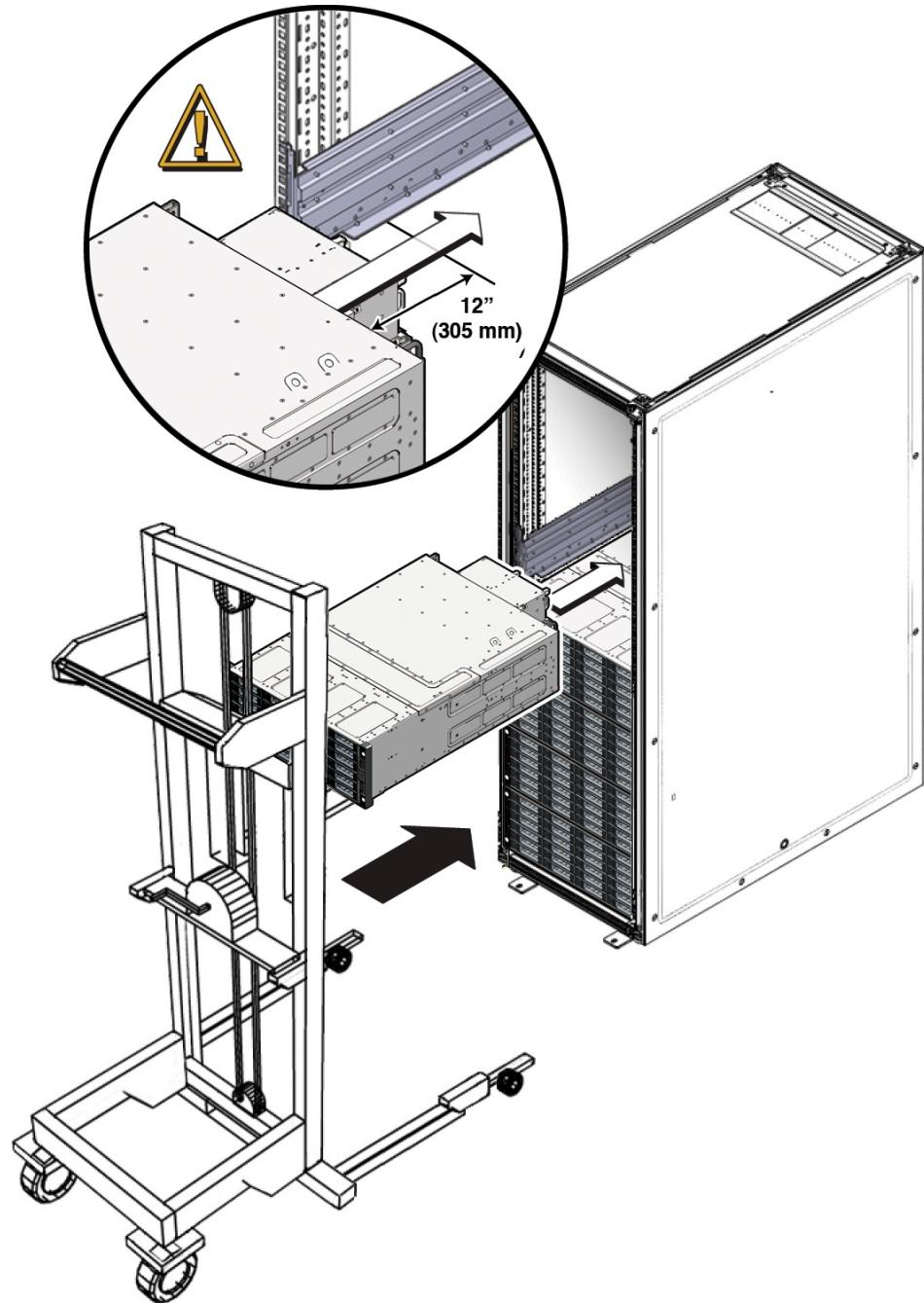
3. Use four screws to attach the front of the system to the front of the rack.
