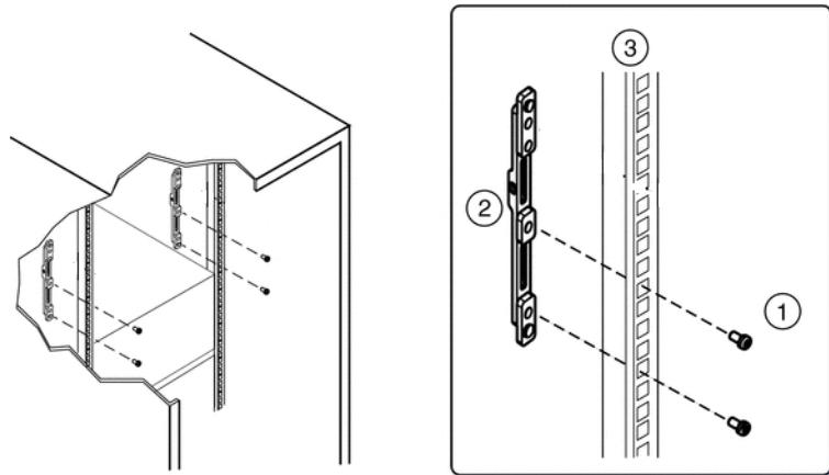
6. Attach rear braces to the rear rack posts and to the adapter brackets.
