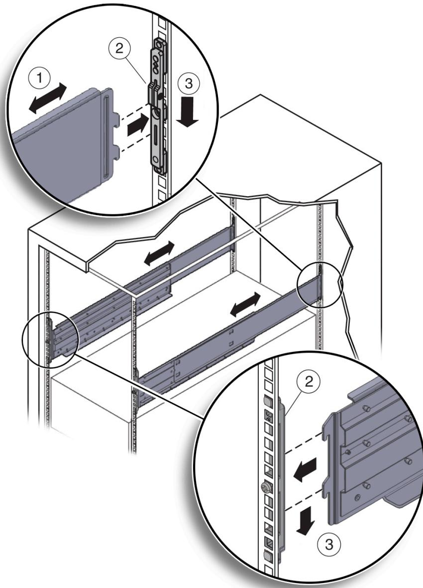
8. Thread the four M4 x 10 flathead locking screws into the four adapter brackets [1].
