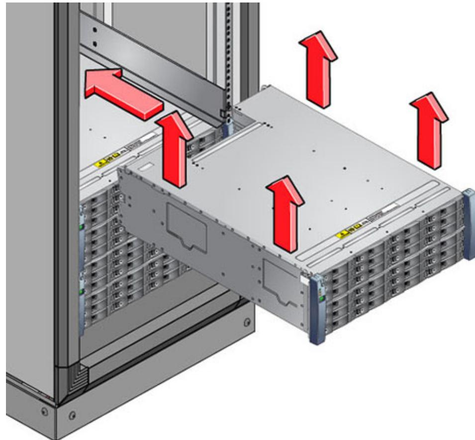
9. Carefully slide the shelf into the cabinet. Ensure that the shelf is fully seated within the rails. If removing the shelf to reseat it, support it at all times.
