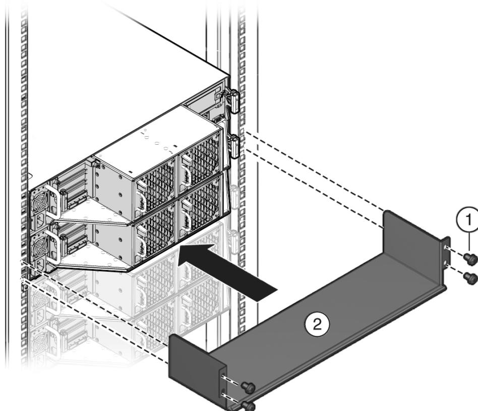
7. Lift the rear shipping bracket up so that it rests firmly against the bottom of the system, then finish tightening the screws that hold the bracket in place.
