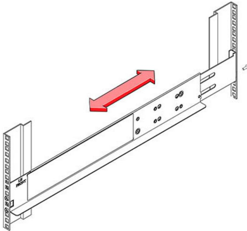
6. Install one screw through the rack and into the rear of each rail.
