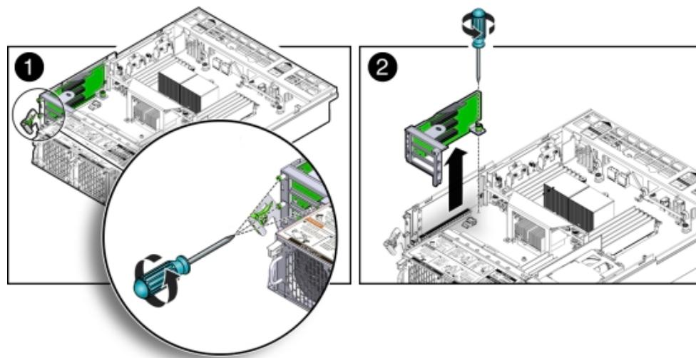
6. Loosen the green captive Phillips screw that secures the PCIe riser to the motherboard [2].
