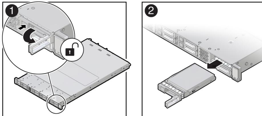
4. Align the replacement drive with the drive slot.
