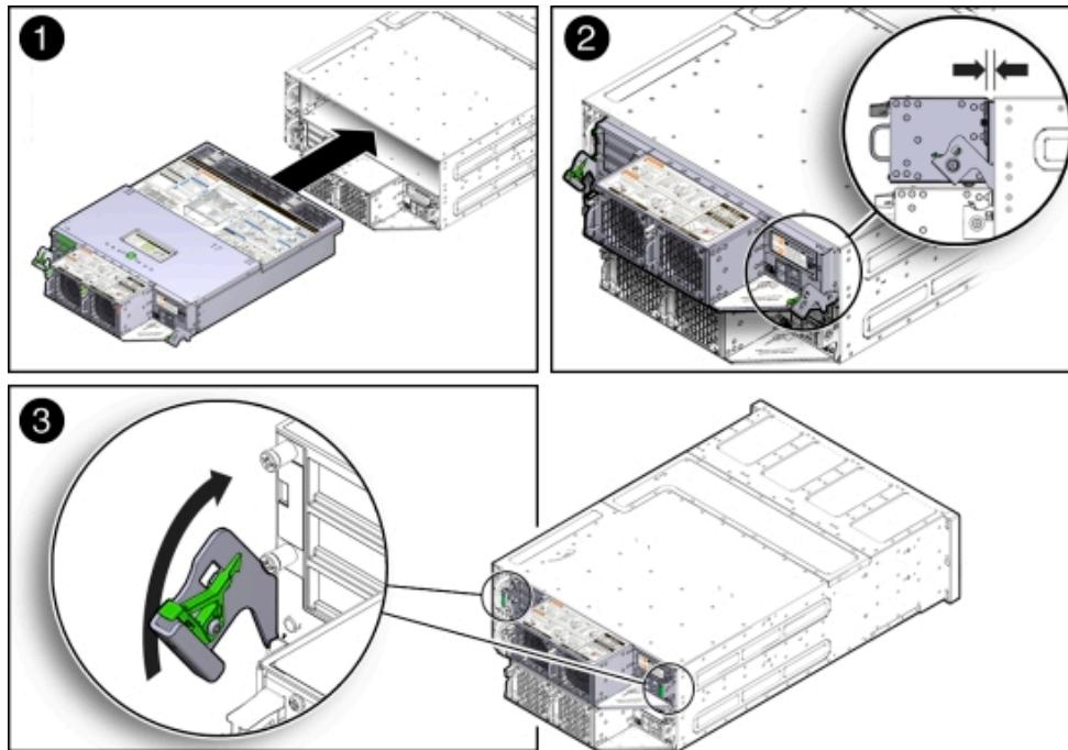
3. To re-seat the server node in the system chassis, grasp both release latches, one on each side of the server node, and push them upward simultaneously to the closed position [3] as shown in the previous figure.
