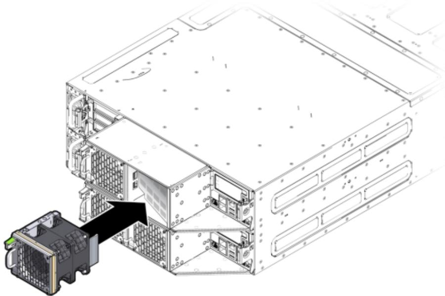
3. Verify that the Fan Fault Status LED on the replacement fan module is lit green.
