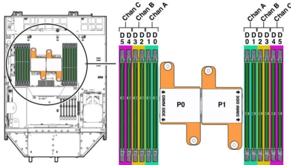
Each processor socket supports three independent memory channels labeled channel A, B, and C, where channel A is closest to the processor socket. Each channel supports two DIMM slots, is controlled by an independent memory controller, and operates independent of the other channels.
