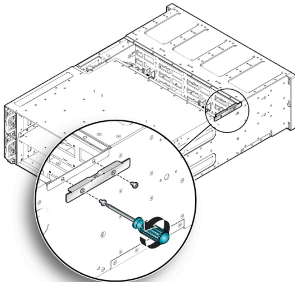
6. Remove the power distribution board.
