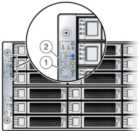
On the server node, the green Power/OK LED (see [2] in the previous figure) blinks while the server node is booting, and remains steady on when the server node is operational.
