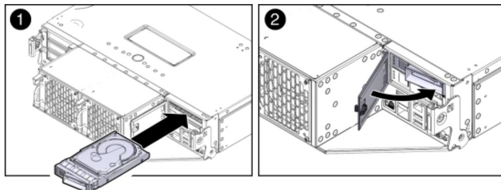
4. Close the drive latch to lock the drive in place.
