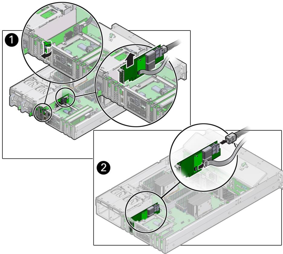
5. Disconnect the super capacitor cable and the SAS cables from the SAS HBA card [2] as shown in the previous figure.
