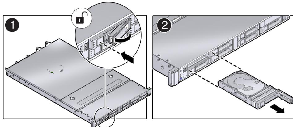
4. Align the replacement drive with the drive slot.
