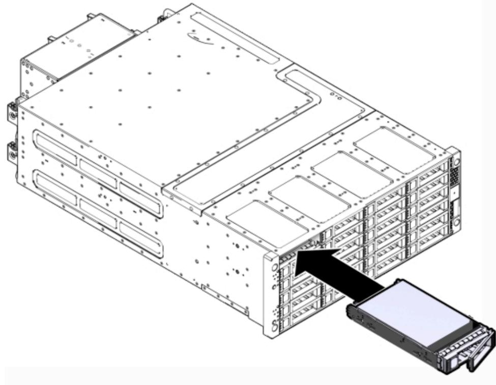
3. Close the latch to lock the drive in place.
