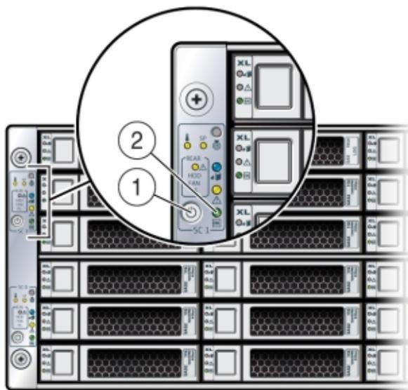
2. To shut down a server node using the Oracle ILOM, perform one of the following:
