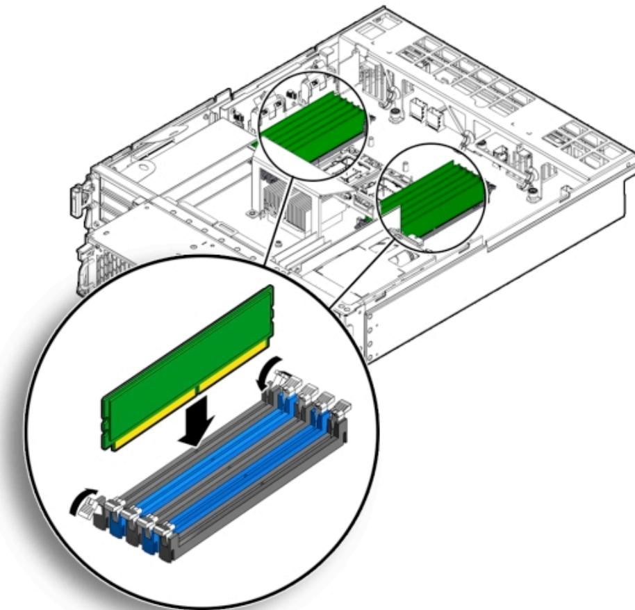
5. Push the DIMM into the connector until the ejector tabs lock the DIMM in place.
