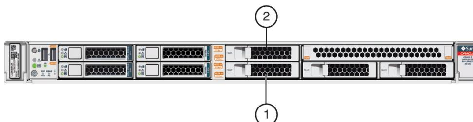
If you have the default configuration of only two NVMe drives (seen as `pd_00` and `pd_01` from the host), you can expand storage by adding two (2) NVMe drives.
