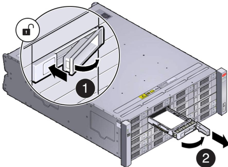
2. b. Open the drive lever of the new drive by pressing the release button on the drive.
