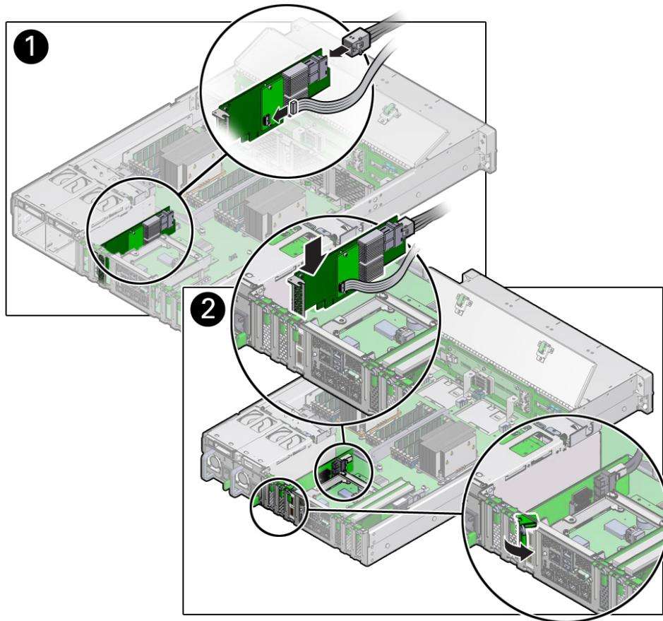
11. Insert the SAS HBA card into PCIe slot 3, and rotate the PCIe locking mechanism to secure the PCIe HBA card in place [2] as shown in the previous figure.
