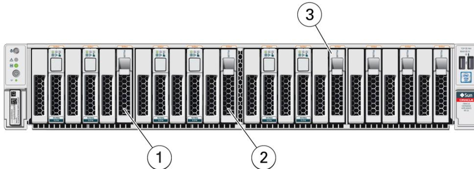
If you have the default configuration of NVMe drives (seen as `pd_00`, `pd_01`, `pd_03`, `pd_04`, `pd_06` and `pd_07` from the host), you can expand storage by adding three (3) NVMe drives.
