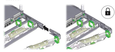
F Remove the tape that secures the slide-rail latching bracket to connector D and ensure that the latching bracket is properly aligned with connector D.
