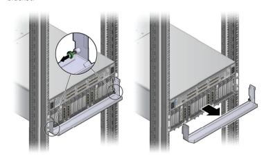
C Carefully pull the bracket away from both Fabric Interconnects, and out of the rack.
