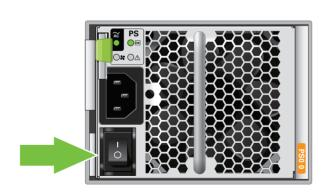
Note: The image shows the circuit breaker on the left power supply.
