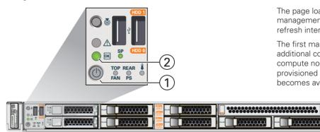
E Wait approximately 5 minutes to allow the management system to power on completely. When complete, the Power/OK LED (2) illuminates and remains a steady green. F On the workstation, browse to the Private Cloud Appliance Dashboard at: http://192.168.4.216.
