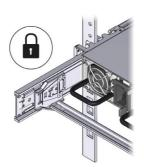
C Insert the CMA's connector B into the front slot on the right slide-rail until it locks into place with an audible click.
