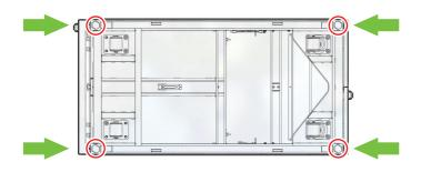
**CAUTION:** If the rack needs to be moved, make sure that the leveling feet are fully retracted and out of the way.
