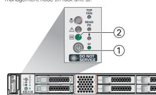
E Wait approximately 5 minutes to allow the management system to power on completely. When complete, the Power/OK LED (2) illuminates and remains a steady green.
