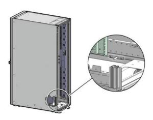
**NOTE:** An additional chassis earth ground cable (not supplied) enables electrical current leakage to dissipate more efficiently.
