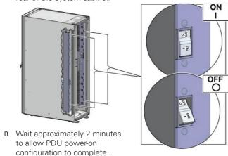
**Note:** Appliance infrastructure components without power switches are powered on together with the PDUs.
