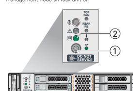
E Wait approximately 5 minutes to allow the management system to power on completely. When complete, the Power/OK LED (2) illuminates and remains a steady green.
