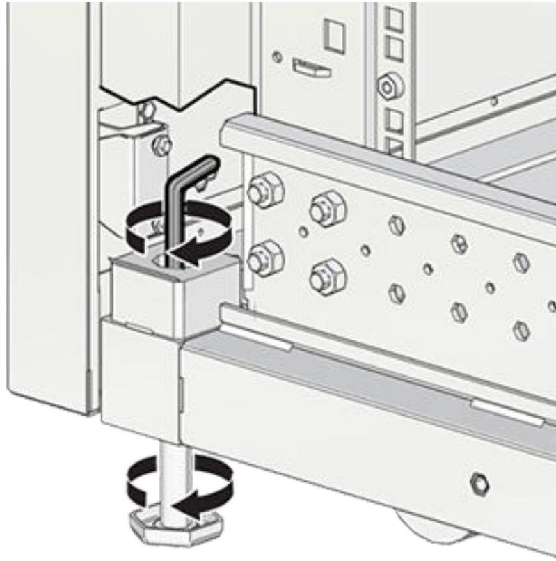
3. Lock the four leveling feet using an 18mm open wrench.
