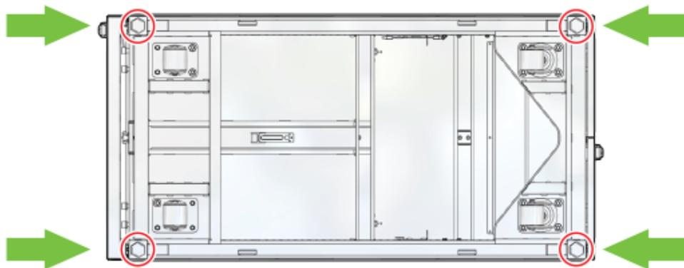
2. Using a 6mm hex wrench, lower the leveling feet to the floor.
