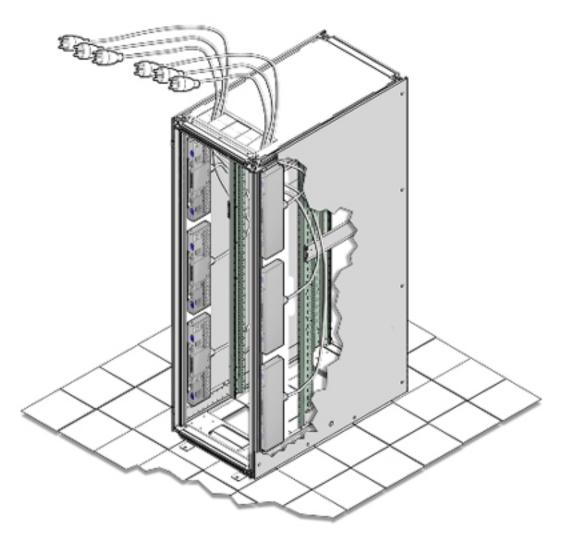
6. Plug the power distribution unit (PDU) power cord connectors into the facility receptacles. Ensure the breaker switches are in the OFF position before connecting the power cables.
