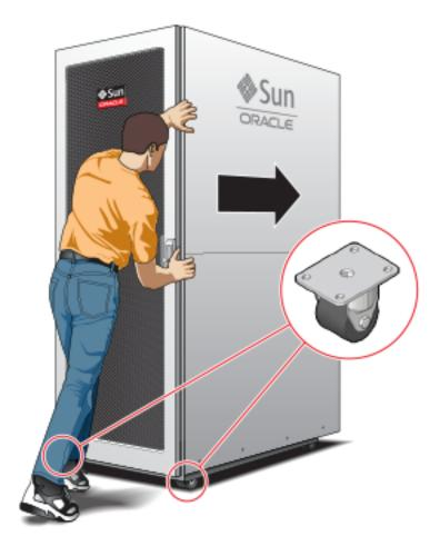
4. When the rack is at the installation site, verify that no components or connections have become dislodged or disconnected during transport. If necessary, re-attach components and cables properly.
