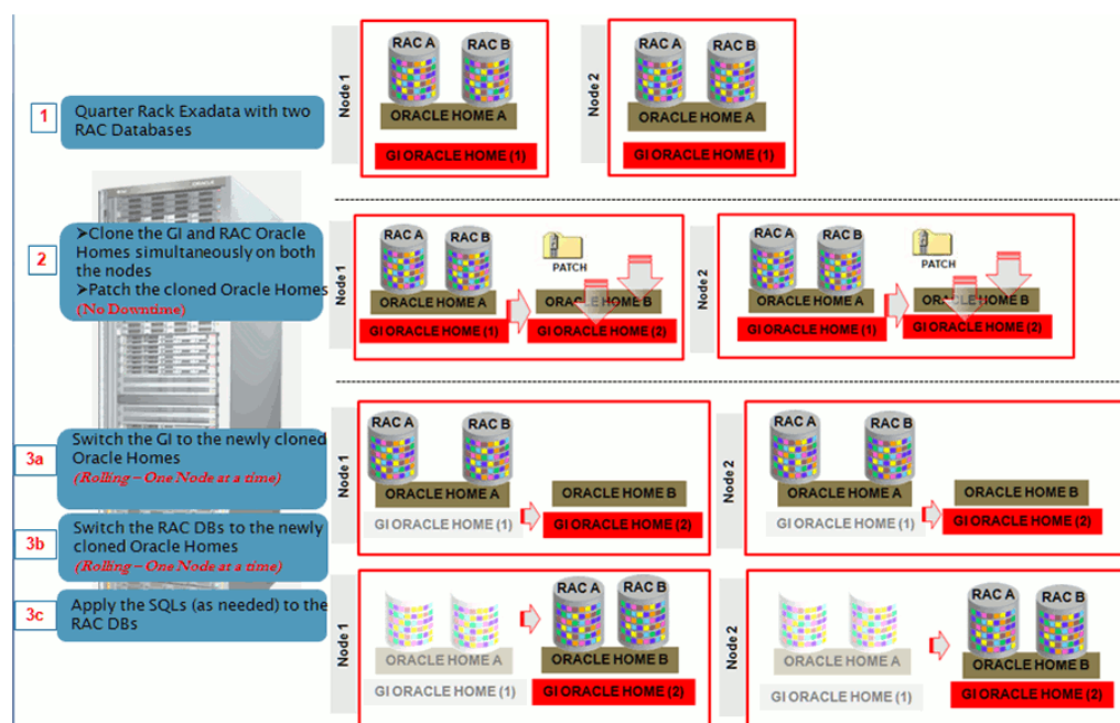
Figure 44-10 Out Of Place Patching Of Clusters
