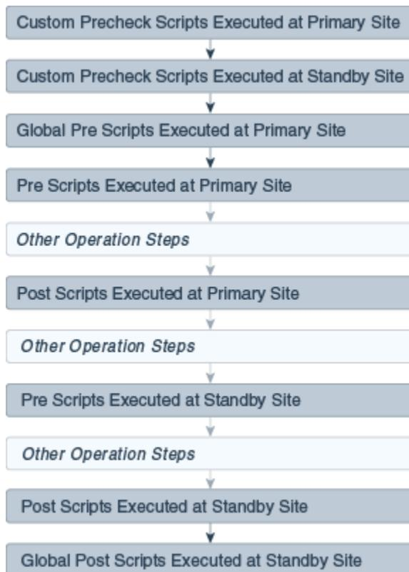
**Figure 2-5 Execution Sequence of Scripts for Failover Operation**
