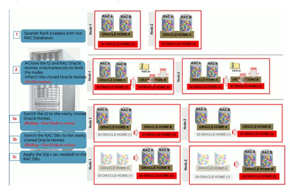
Figure 14-8 Out Of Place Patching Of Clusters
