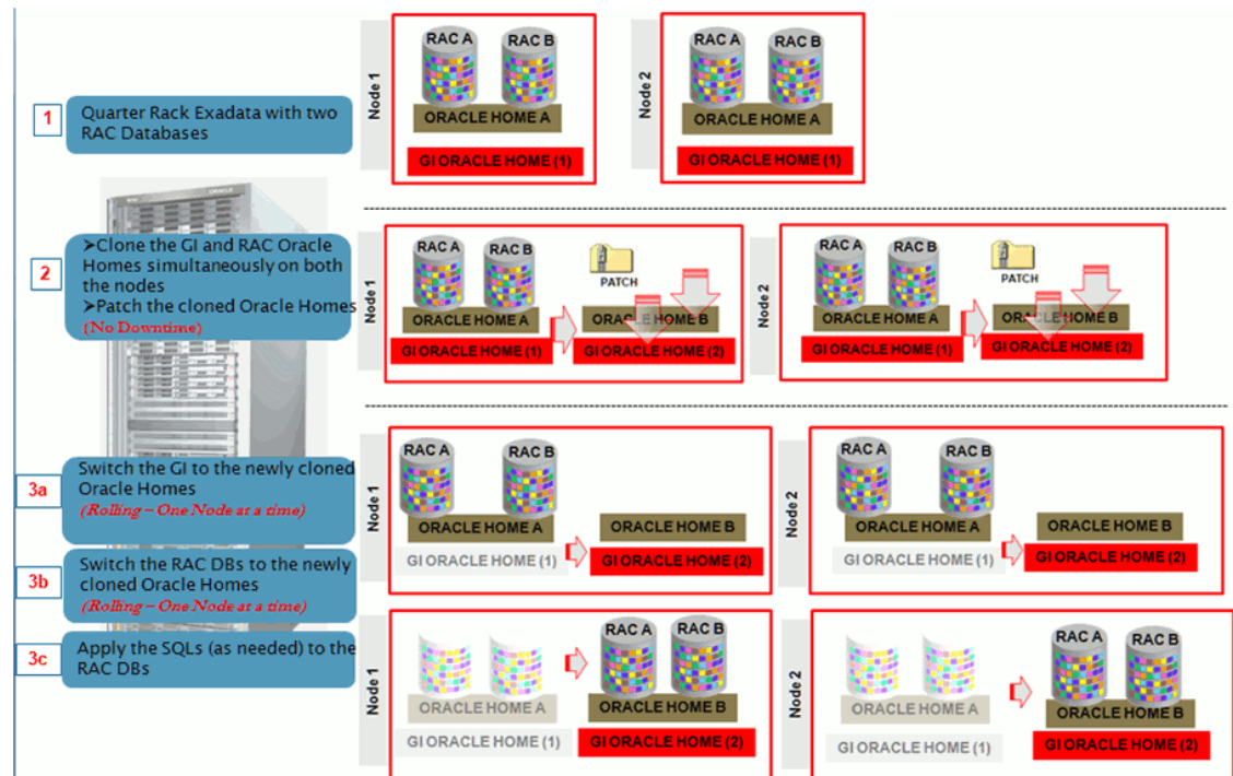
Figure 8-8 Out Of Place Patching Of Clusters
