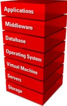
The Enterprise Manager Systems Infrastructure (EMSI) plug-in is a fully integrated software plug-in that provides monitoring and an enterprise-wide view the bottom half of the stack, including Oracle Solaris and Linux operating systems, virtualized operating systems (zones) and virtual machines (logical domains), servers, storage appliances, storage for a host, and network resources.
