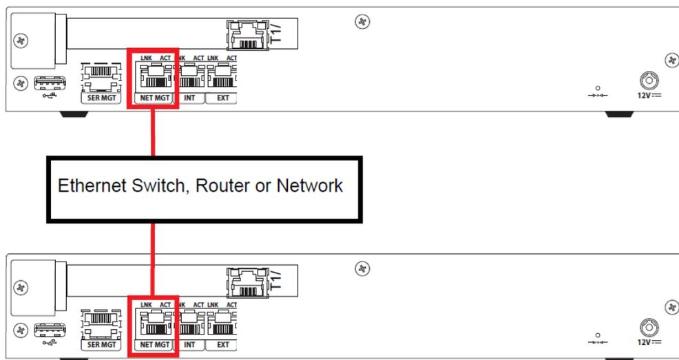
To cable the Acme Packet 1100 in an HA configuration using single rear interface support:
