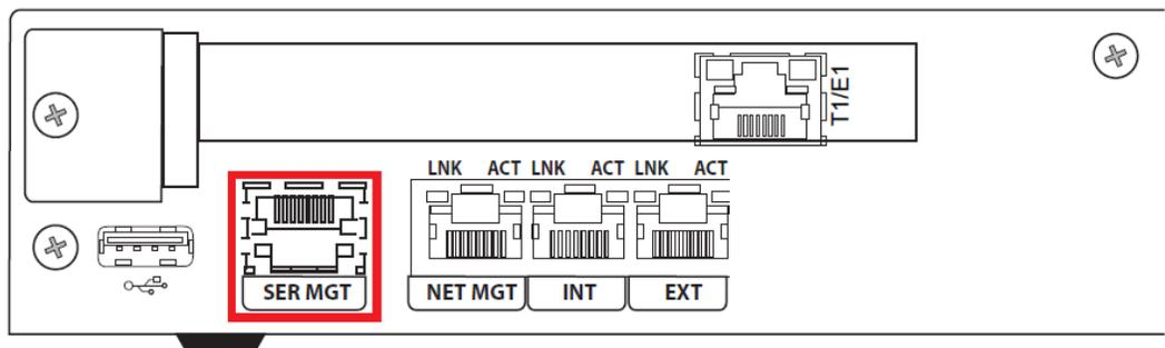
2. Insert the RJ45 connector on the end of the console cable into the console port labeled SER MGT.
