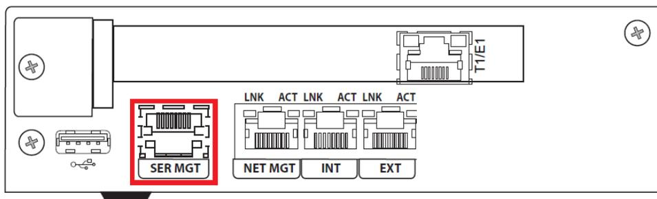
3. If the Acme Packet 1100 is already powered on, press Enter a few times to activate the console connection. When ACLI text is displayed on the screen, the console connection has been successfully created.
