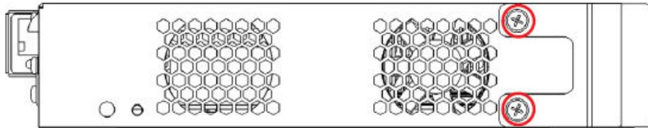
3. Attach the rack mount flange to the chassis as shown by inserting a #6-32 x 5/16" screw into each of the holes, and use a Phillips screwdriver to hand-tighten and secure each screw.
