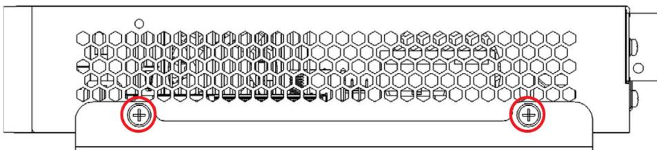
3. Insert a #6-32 5/16" screw and washer into each of the holes and then use a Phillips screwdriver to hand-tighten each screw to secure the wall bracket to the chassis.
