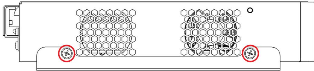
5. Insert a #6-32 5/16" screw and washer into each of the holes and then use a Phillips screwdriver to hand-tighten each screw to secure the wall bracket to the chassis.
