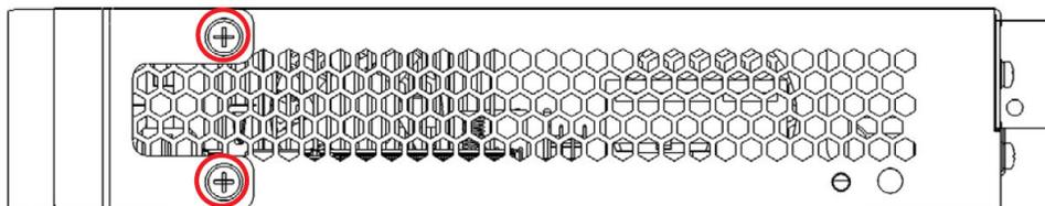
5. Attach the rack mount flange to the chassis as shown by inserting a #6-32 x 5/16" screw into each of the holes and then use a Phillips screwdriver to hand-tighten and secure each screw.
