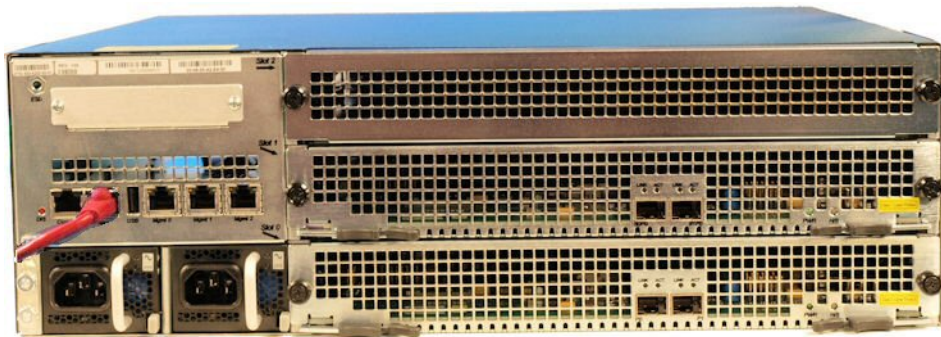
Connected Alarm Port Cable
