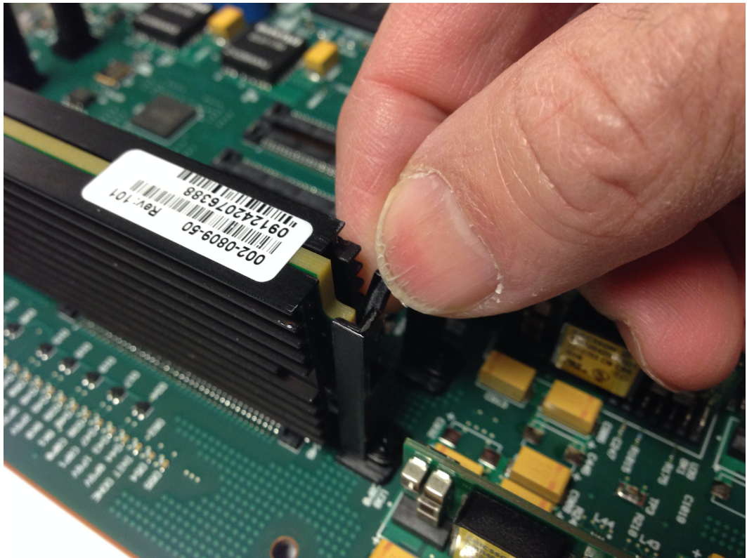
Releasing the Fastener Holding the TM (1 of 2)
