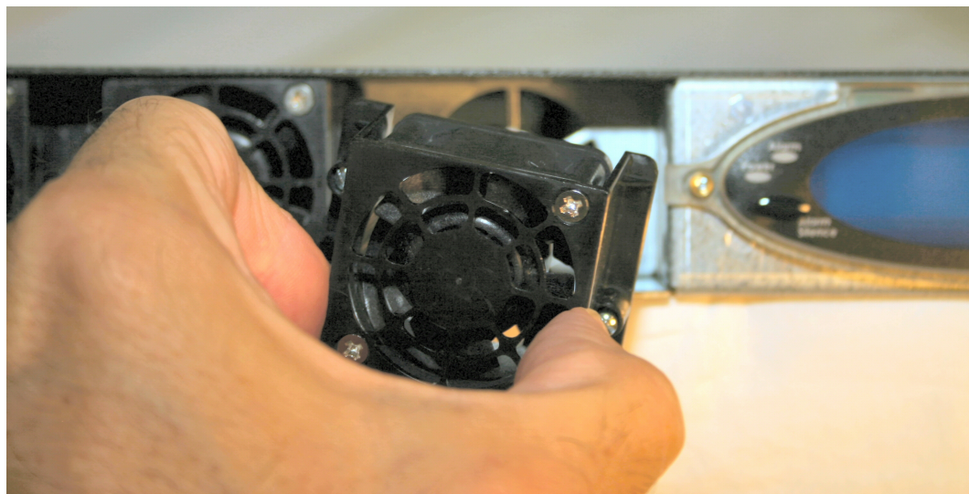
Figure 6-5 Inserting the Fan into the Chassis Slot
