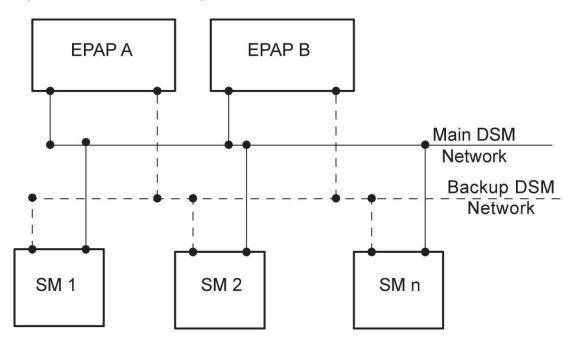
Figure 2-7 DSM Provisioning Task Interfaces
