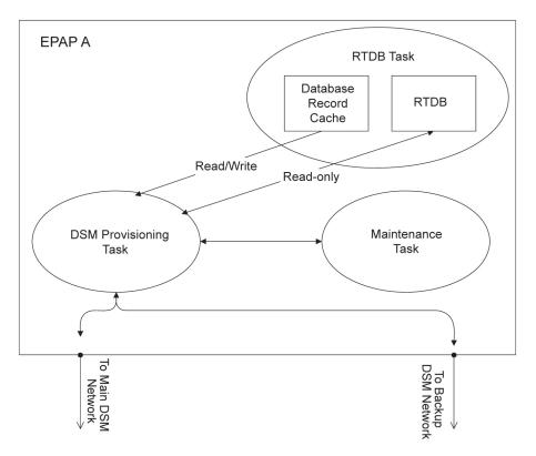
In order to handle the redundancy requirements for this feature, a separate RMTP channel is created on each interface from each EPAP:
