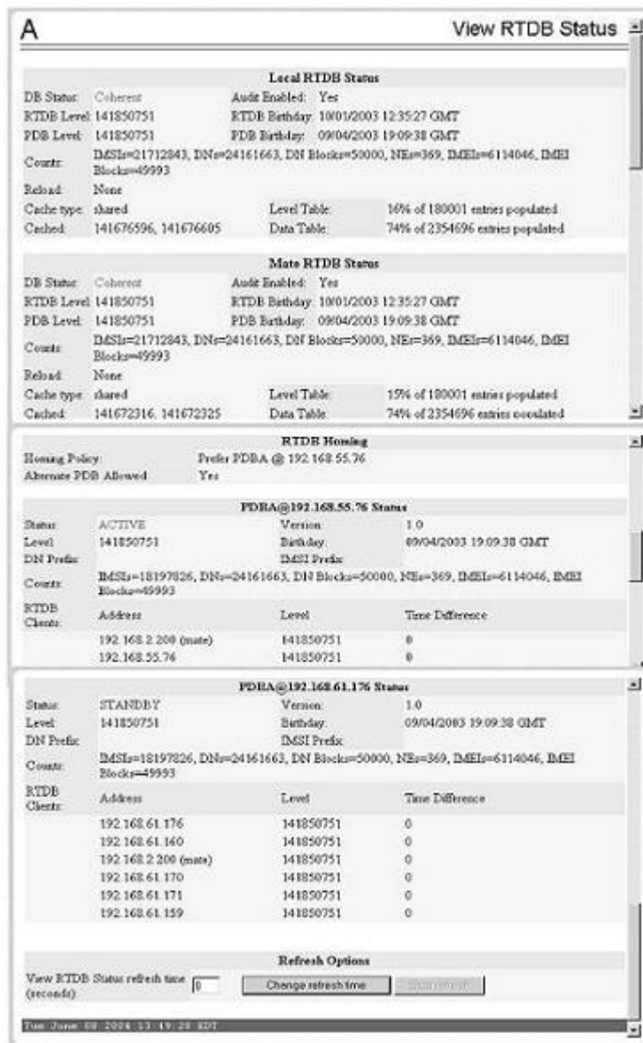
Figure 3-37 View RTDB Status Screen
