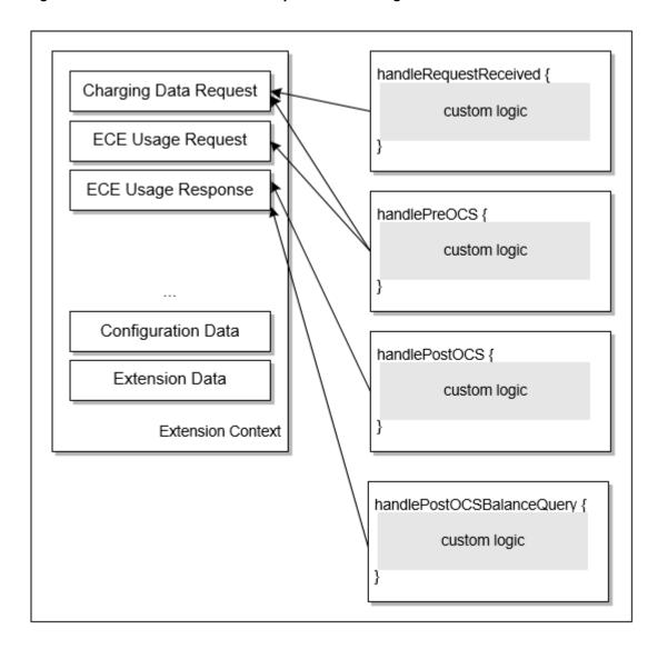
Figure 23-8 Data Used in HTTP-Request Processing Extension Points
