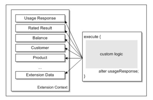
Figure 23-14 Data Used in Post-Charging Extension Point
