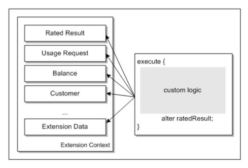
Figure 23-13 Data Used in Post-Rating Extension Point
