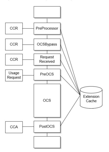
Figure 23-1 Diameter-Request Processing Extension Points
