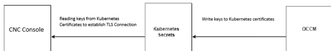
Figure 2-4 Establishing Connection Between CNC Console and TLS Using OCCM Key
