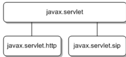
Figure 2-1 HTTP/SIP Convergence in the SIP Servlet API
