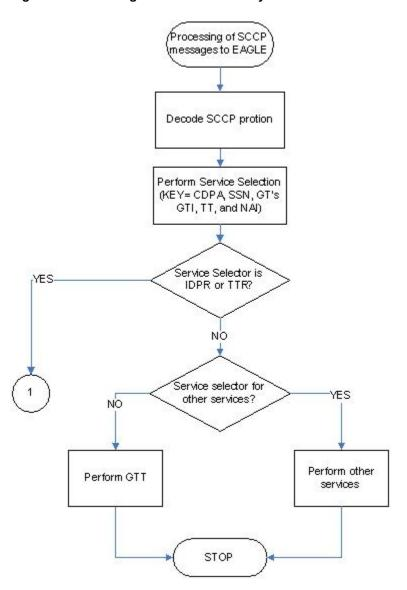
Figure 2-1 Message Flow for IDP Relay - Sheet 1 of 3
