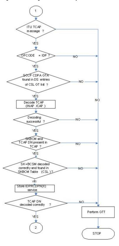
Figure 2-2 Message Flow for IDP Relay - Sheet 2 of 3
