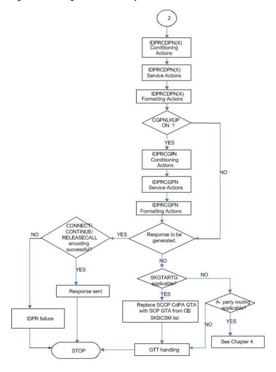
Figure 2-3 Message Flow for IDP Relay - Sheet 3 of 3
