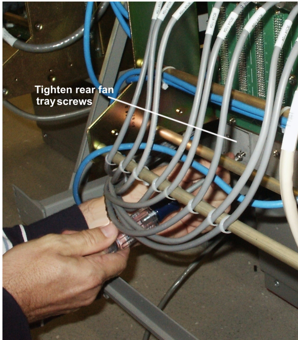
Figure 6-21 Tighten rear fan tray screws
