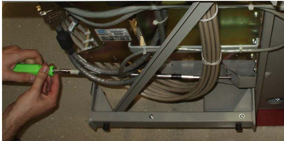
Figure 6-22 Tighten fan side bracket screws
