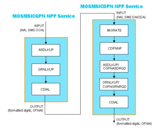
Figure 2-10 MO SMS NPP - IS41 Processing
