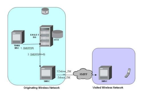
Figure 2-4 MO-Based IS41 SMS NP Call Flow for Other-Network Subscriber
