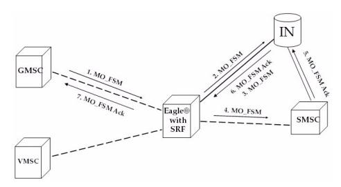
Figure 2-6 Successful Delivery of Mobile Originated FSM from Prepaid Subscriber
