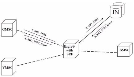
The Gateway Mobile Switching Center (GMSC) sends the Mobile Originated Forward Short Message (MO\_FSM) to the EAGLE with PPSMS (TCBEGIN). Based on MTPDPC = EAGLE point code and SCCP CdPA TT, NP, NAI, and GTI, the message is pre-selected for PPSMS service. If service is not PPSMS, the message falls through to GTT.
