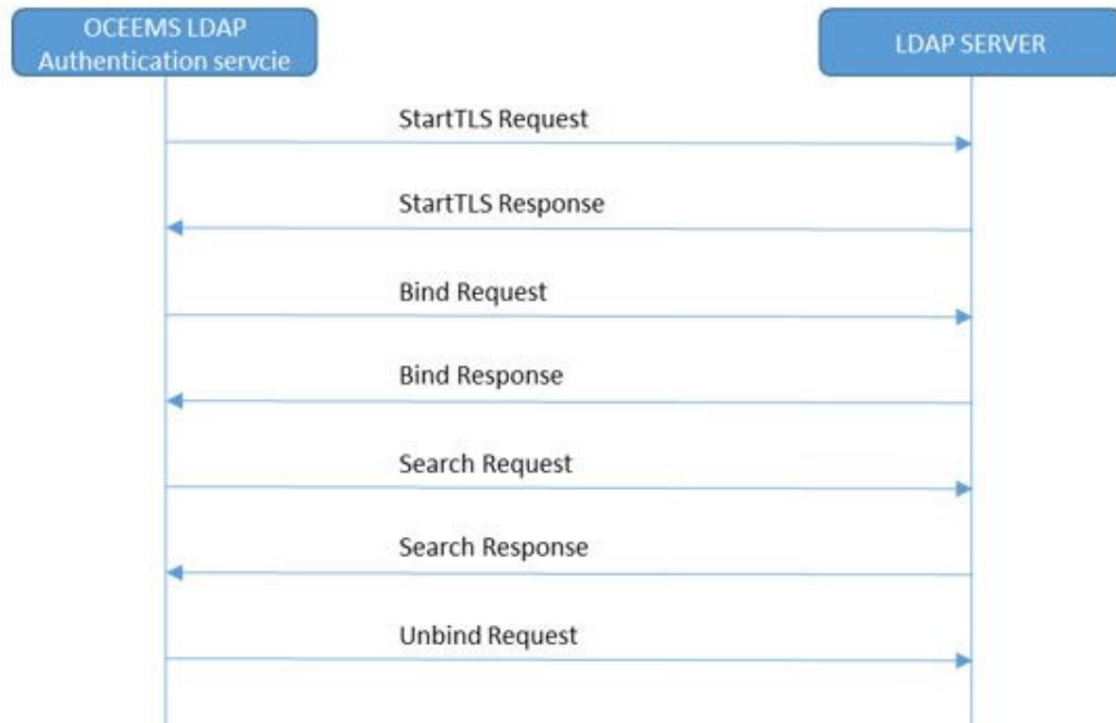
Figure 7-1 Sample Call Flow for LDAP Authentication
