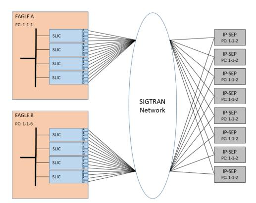
Figure 5-4 Mated Signaling Transfer Point Redundancy With 4-Port SLIC Cards
