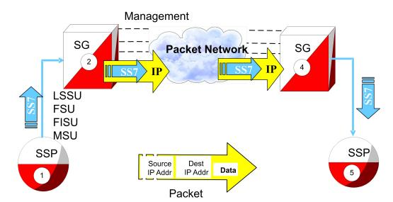
Figure 2-3 Transmitting an SS7 Message using IP
