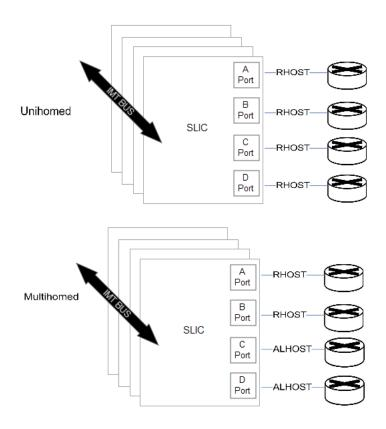
Multi-homing can be used for M2PA links if the M2PA linkset has only one link.
