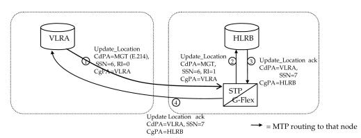
Figure 2-1 E.214 (E.212) Routing Example - Location Updating
