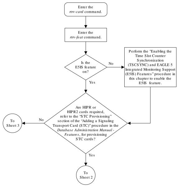
Figure 4-6 Adding a Signaling Transport Card (STC)
