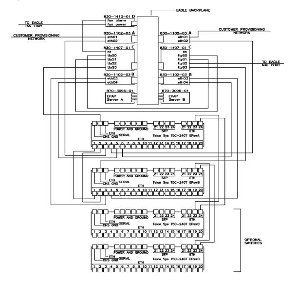
Figure A-1 EPAP Network Connections
