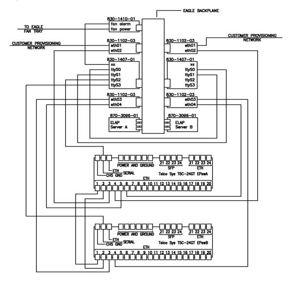
Figure A-4 ELAP Network Connections
