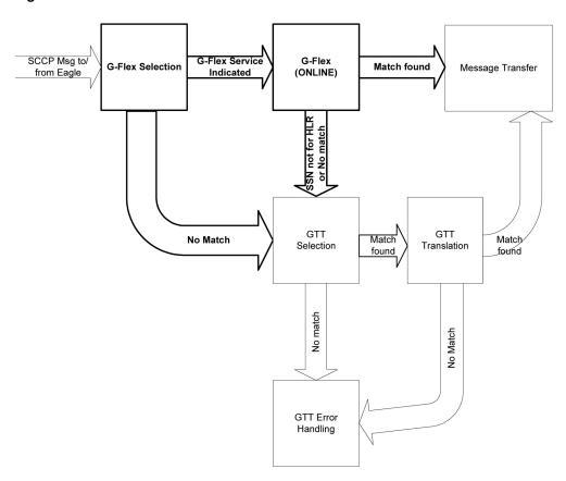
In order to keep the diagram simple, the only error conditions shown are the no-match cases for G-Flex and GTT selectors and translations. G-Flex has its own error handling for some cases that issues UIMs and peg measurements appropriately before letting the **MSU** fall through to GTT translation. Also, there are error conditions in GTT selection, GTT translation, and message transfer that are handled by GTT error handling.
