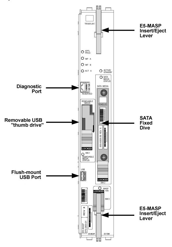
The -02 E5-MASP card has different hardware than the E5-MASP -01 card.
