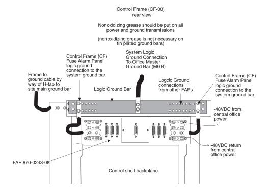
Figure 5-2 Logic Grounding with FAP (P/N 870-1606-xx/870-2320-xx)
