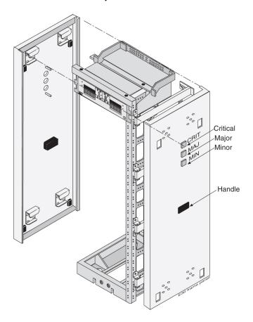
Figure 3-5 Frame End Panel with Lamp Indicators
