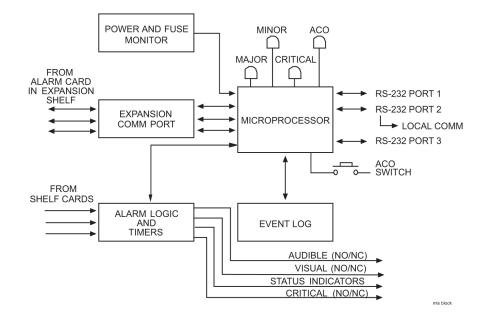
Figure 3-51 Maintenance Interface System Card Block Diagram
