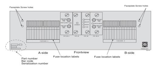
Figure 3-47 Fuse and Alarm Panel (P/N 870-1606-xx/870-2320-xx) Front
