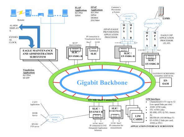
The EAGLE hardware platform consists of various frame types. Each frame holds shelves or rack mounted equipment. The shelves hold the plug-in application and interface cards. Hardware Descriptions - EAGLE provides detailed information about component requirements and hardware configuration.
