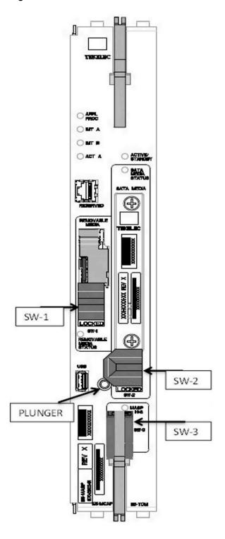
SW-1: Used to activate or de-activate Removable USB "thumb drive." The locked position activates the switch.
