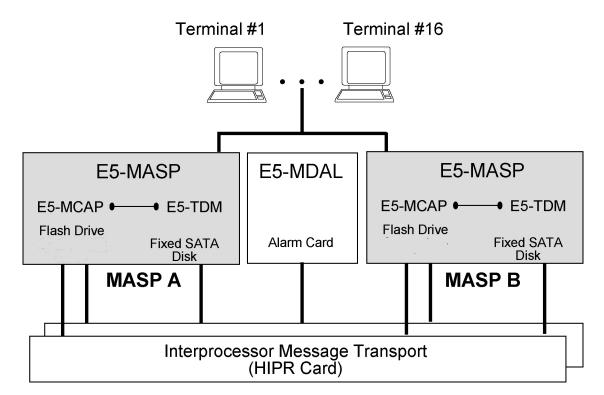
Figure 2-2 E5-based Maintenance and Administration Subsystem Block Diagram
