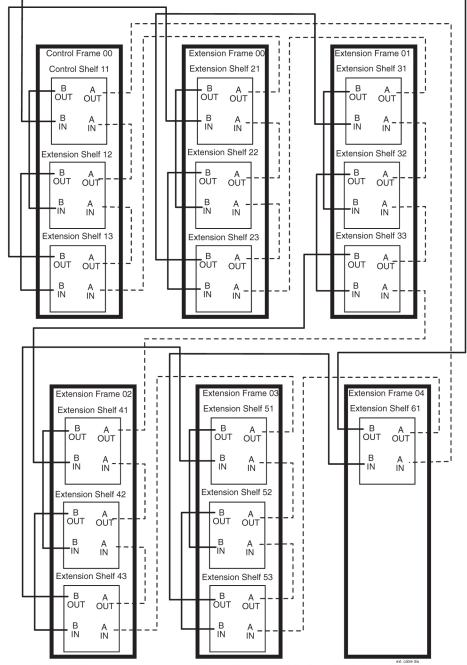
Figure 6-3 Six-Frame Configuration
