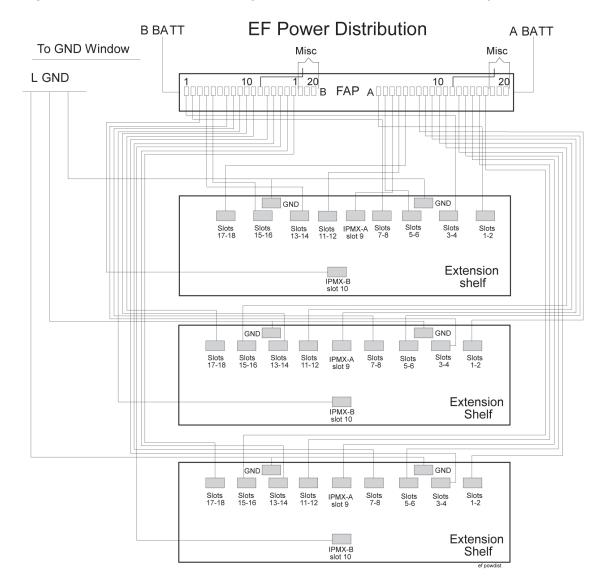
Figure 5-29 Extension Frame FAP (P/N 870-0243-08 and P/N 870-1606-xx)
