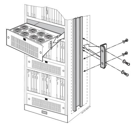
Secure the fan unit with the same screws that were removed from the frame holding the baffle in place.
