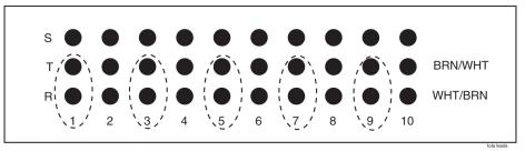
Note: Master Timing leads can only be terminated on the ODD ports on the Holdover Clock Interface Panel. Do not wire on the sleeve pin.
