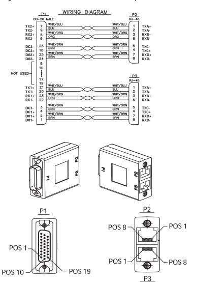
Figure C-5 DB26 Male to Dual RJ45 Adapter
