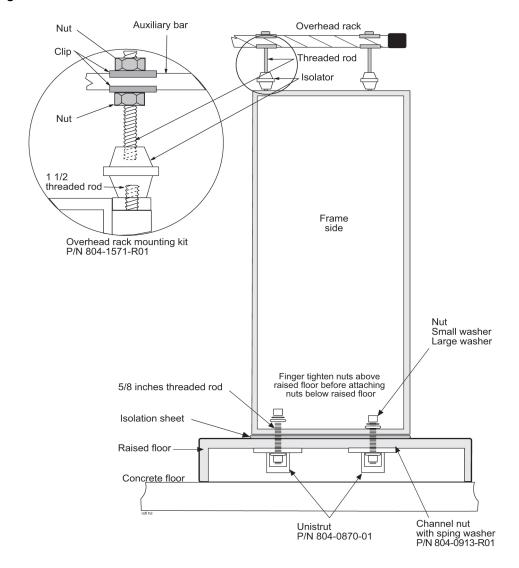
Figure 4-11 Raised Floor Installation With Unistrut
