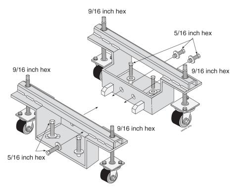
11. Remove the bolts, front and rear, that attach the dolly to the frame. Refer to Figure 4-5.
