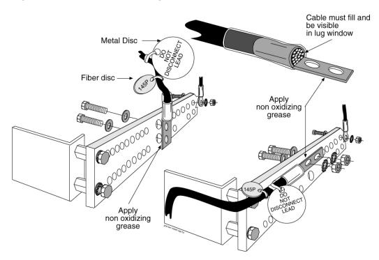
Figure 5-24 Ground Bar and Logic Ground Installation
