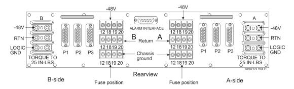
Figure B-5 Alarm Interface Connector
