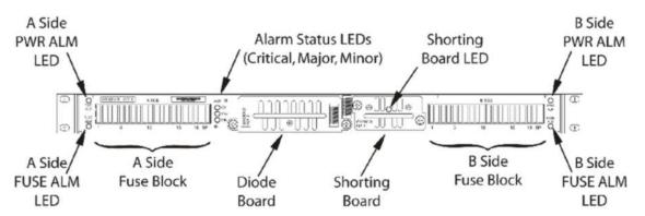
Figure 5-2 Fuse and Alarm Panel - Front View (P/N 870-2804-xx)
