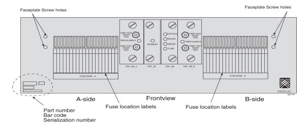
Figure 5-8 Fuse and Alarm Panel (P/N 870-1606-xx/870-2320-xx) Front
