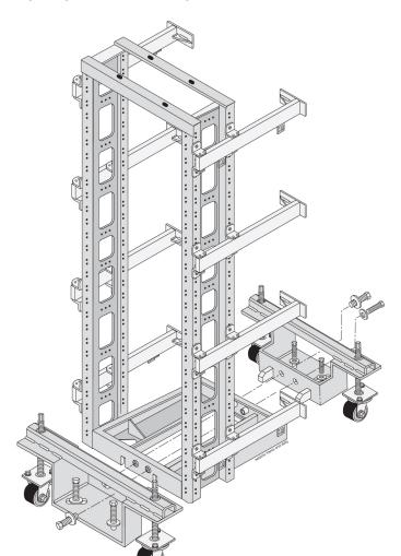
Figure 4-5 Heavy Duty Frame with Dolly
