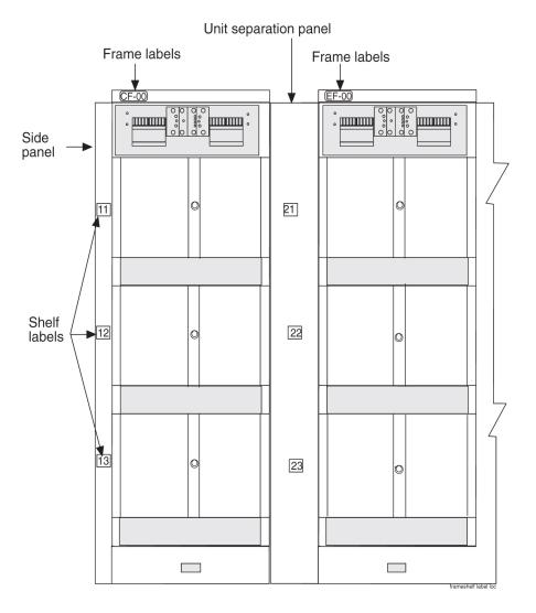
Figure 4-25 Frame Label Location - Detail
