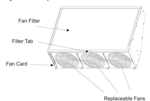
12. Insert the fan tray into the fan tray bracket. You might need to tilt the fan tray up as it is pushed in so that it is completely inserted into the bracket. After insertion, be sure the front of the fan tray is recessed in 1/2 inch with respect to the front frame rails.
