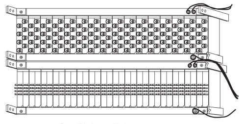
Rear 120 ohms to 75 ohms converter
