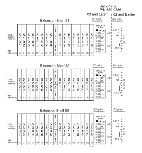
Figure 5-35 Extension Frame EF-04 Numbering Plan
