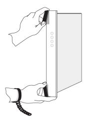
Part number, **LEDs**, text and bar code (**CLEI** and serial number) are located on the faceplate of each card. The cards in the frames are configured with specific functions and services.
