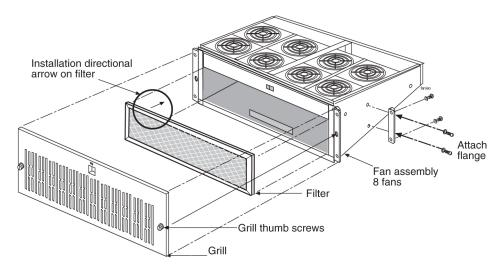
7. Install the fan unit in the space left by the baffle.
