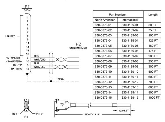
19. Connect P1 of the high-speed source and composite clock cable (P/N 830-0873-xx or P/N 830-1189-xx) connector end to the appropriate ckock connector(J48 or J49). Tighten the connector with a slotted screw driver.
