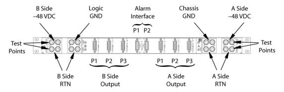
Figure 5-23 3U Fuse and Alarm Panel Rear (P/N 870-2320-03))
