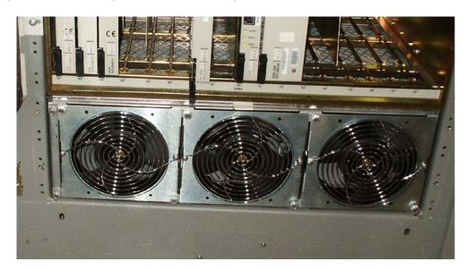
13. When the fan tray is aligned and in place, attach the fan tray to the fan tray bracket by tightening the screws on the left and right sides of the rear of the fan tray bracket. There are two screws on each side. These screws must be tightened from the rear of the frame.
