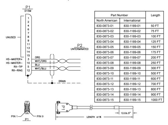
11. Connect P1 of the high-speed source and composite clock cable (P/N 830-0873-xx or P/N 830-1189-xx) connector end to the appropriate IDLE ckock connector(J48 or J49). Tighten the connector with a slotted screw driver.
