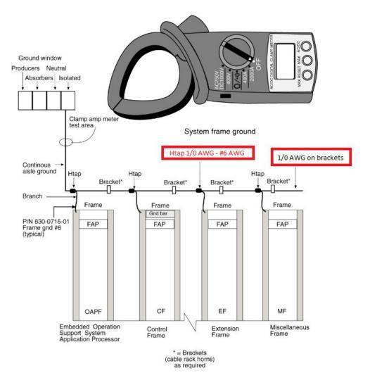
Figure 5-17 System Frame Grounding
