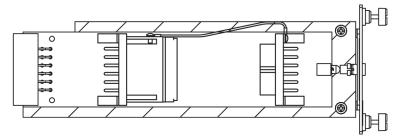
**4.** Slide the jumper board back into the **FAP**. Verify the **OP/MAINT LED** lights green. The fuse alarm **LED** returns to green.
