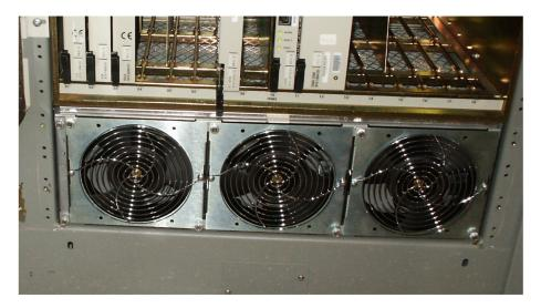
3. When the fan unit is aligned and in place, attach the fan unit to the fan tray bracket by tightening the screws on the left and right sides of the rear of the fan tray bracket. There are two screws on each side. These screws must be tightened from the rear of the frame.
