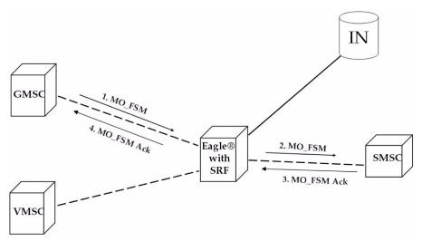
The Gateway Mobile Switching Center (GMSC) sends the Mobile Originated Forward Short Message (MO\_FSM) to the EAGLE with PPSMS (TCBEGIN).
