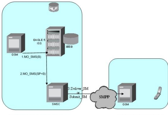
Figure 2-2 MO-Based GSM SMS NP Call Flow for Other-Network Subscriber
