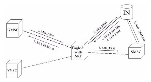
The Gateway Mobile Switching Center (GMSC) sends the Mobile Originated Forward Short Message (MO\_FSM) to the EAGLE with PPSMS (TCBEGIN).
