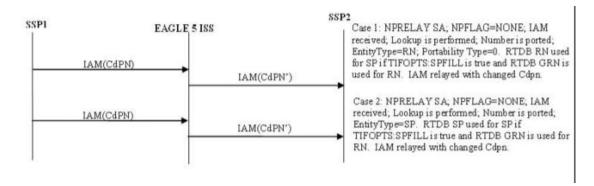
A use case using both the NPRLS and NPRELAY Service Actions is shown in the following figure. In this example, only OLO subscribers are released; own-network subscribers are relayed. The Service Actions would be set to NPRLS and NPRELAY. The NPTYPERLS configuration option is set to RN and the NPTYPERLY configuration option is set to SP.
