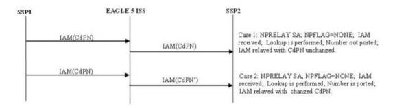
The following figure shows TIF NP Relay cases where NM bits are used in the ISUP IAM message. In the sequence diagrams, the NM bits are shown as binary values. Refer to <u>Use of NM Bits</u> for details on the use of NM bits.
