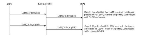
A TIF NP CgPN use case is shown in the following figure for a TIFCGPN, TIFCGPN2, or TIFCGPN3 NPP service when NPRELAY (in TIF, TIF2, or TIF3) and CGPNNP (in TIFCGPN, TIFCGPN2, or TIFCGPN3) Service Actions are provisioned and RTDB lookup is performed on both CdPN and CgPN. A TIFCGPN, TIFCGPN2, and TIFCGPN3 NPP service is invoked by the corresponding TIF, TIF2, or TIF3 NPP Service.
