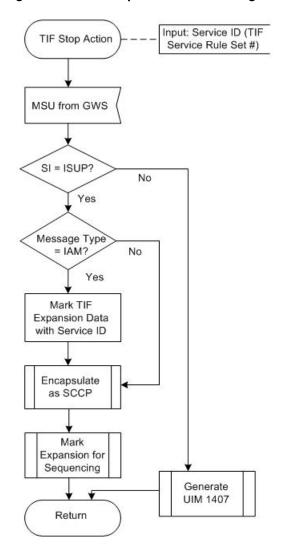
Figure 2-2 TIF Stop Action Processing
