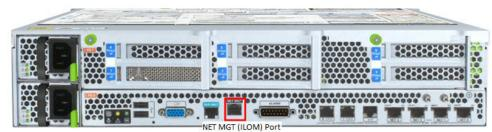
3. Lead the cable away from the rear panel, and connect the other end of the cable to the LAN.
