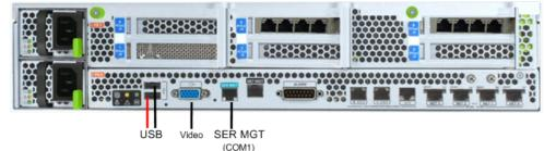
Connecting to USB, VGA and SER MGT (COM1) Ports
