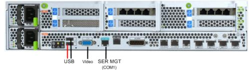
Connecting to USB, VGA and SER MGT (COM1) Ports
