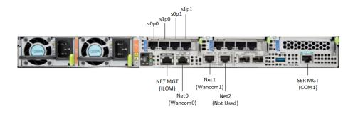
Figure 1-12 Oracle X8-2 Configuration B (Two 4x10 GigE NICs)
