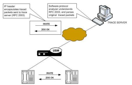
It is possible that—for large frames—when the Oracle® Enterprise Session Border Controller performs the steps to comply with RFC 2003 by adding the requisite header, the resulting packet might exceed Ethernet maximum transmission unit (MTU). This could result in packets being dropped by external network devices, but widespread support for jumbo frames should mitigate this possibility.
