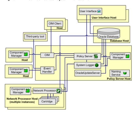
Figure 1-1 IP Service Activator System Architecture
