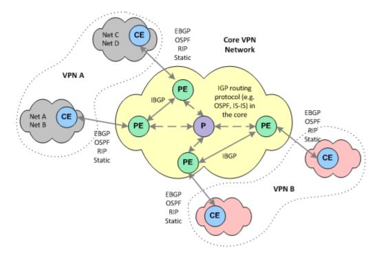
Figure 4-3 MPLS VPN Routing Protocols
