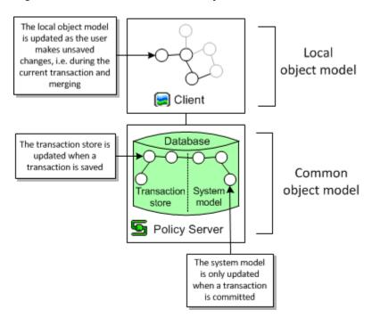
Figure 3-4 Local and Common Object Models
