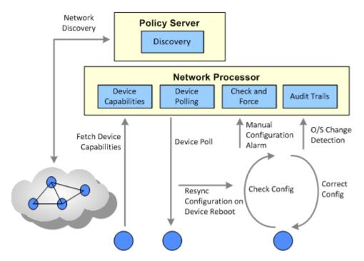
Figure 2-3 Techniques for IP Service Activator Device Integrity
