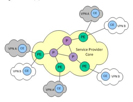
The Service Provider is responsible for managing the backbone, comprising the PE and the P routers. From an MPLS point of view, all routers in the core are LSRs. The PE devices are edge LSRs, responsible for attaching label headers at ingress and stripping labels at egress.
