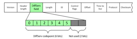
The six DiffServ bits allow the definition of up to 64 different classes of service. However, the standards define a number of recognized codepoint settings and the corresponding packet forwarding treatment, known as a per-hop behavior.
