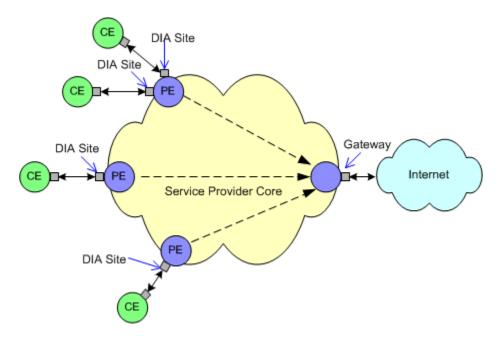
A Layer 3 interface is configured or created and placed in a DIA site. In a managed CE service, the CE device is also placed in the DIA site. IP routing is configured on the PE to route Internet traffic across the provider core to the Internet gateway and on to the Internet. Additionally, prefix lists may be configured to filter routing updates.
