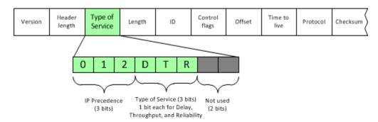
The three-bit IP Precedence field is intended to indicate the importance or priority of the packet. It allows a set of eight values from 0 to 7 to be set, where 0 is the lowest priority and 7 is the highest. Values 6 and 7 are normally reserved for network control traffic, such as routing updates, leaving six values available for normal traffic.
