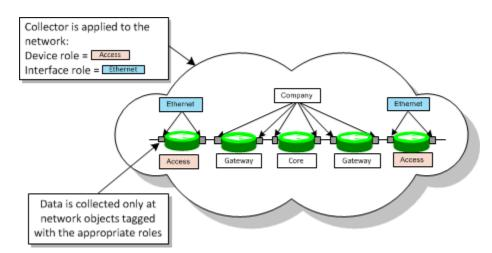
Figure 4-1 Collectors and IP Service Activator Device Roles
