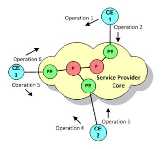
Figure 2-7 Two-way Probes in a Fully-Meshed VPN
