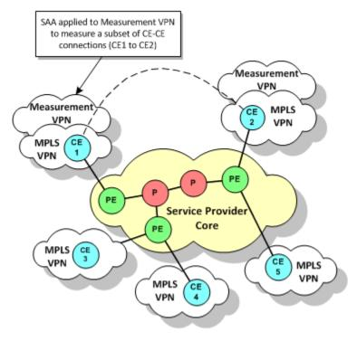
Figure 2-9 Measurement-only VPN Overlay
