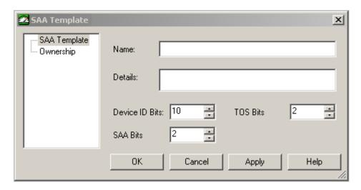
By adjusting the values of Device ID Bits, TOS Bits, and SAA Bits, you can increase the number of devices within the VPN, the number of operations, or the number of operation types that can be applied. The values specified for these three fields must add up to exactly 14. If you choose to increase the number of bits allocated to the device ID, you must reduce either the number of bits allocated to the ToS value or the SAA operation type.
