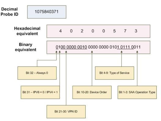
Table 2-1 Components of the SAA Probe Calculations
