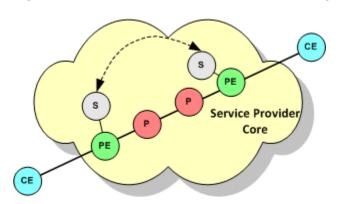
Figure 2-12 SAA for PE to PE Connections using Shadow Routers
