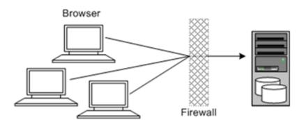
Figure 1-2 Single-Computer Deployment Topology
